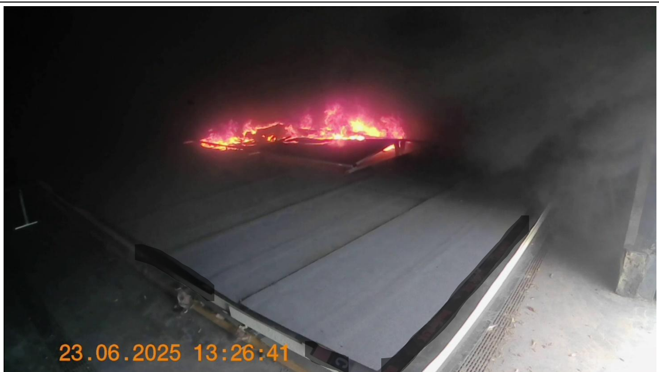
Figure 19: Solar panel diagonally across from gas burner fully involved (Camera 1)
