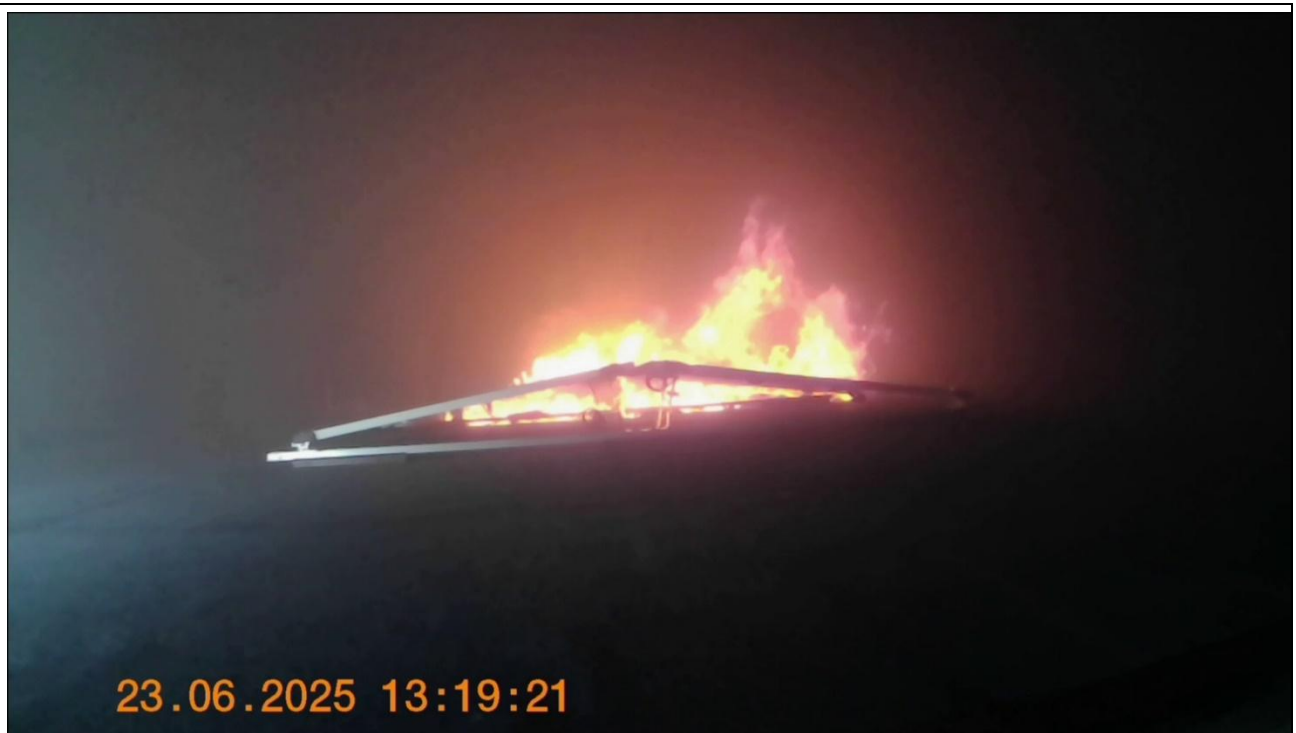
Figure 17: Roof assembly begins to catch alight (Camera 3)
