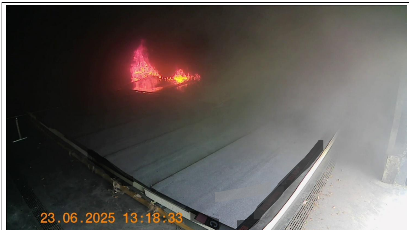
Figure 15: Solar panel above gas burner fully involved (Camera 1)
