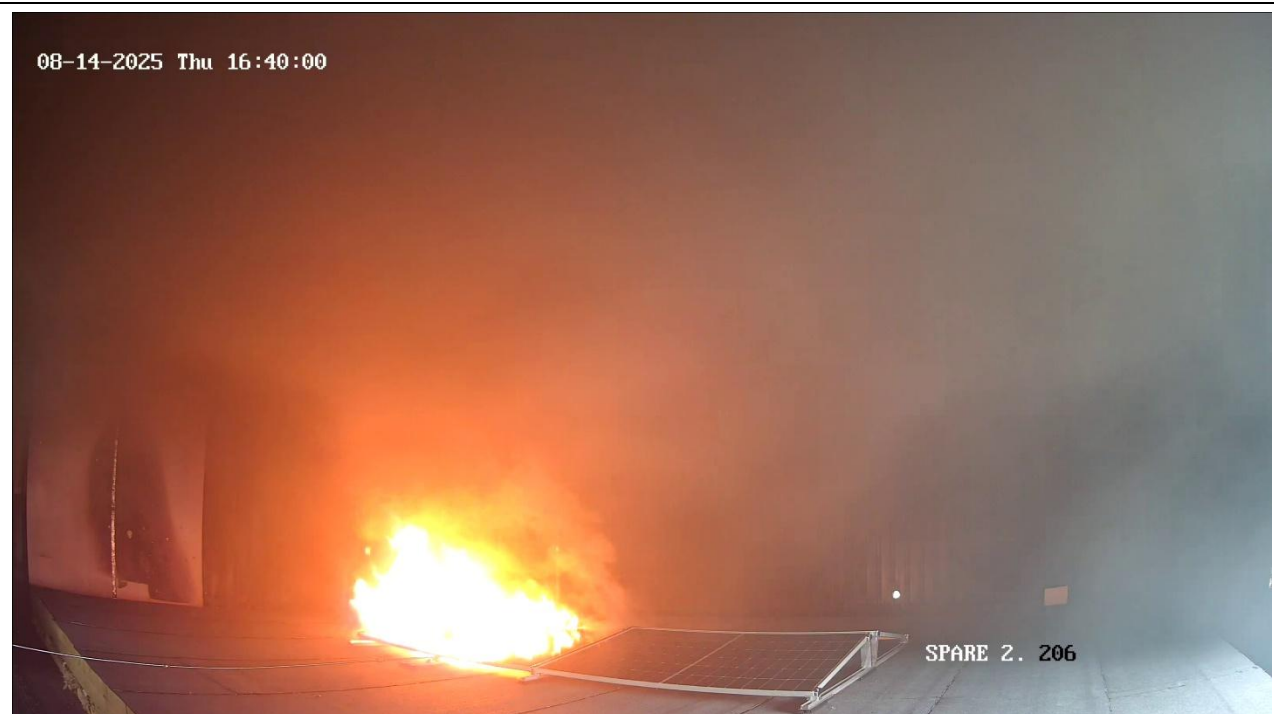
Figure 37: Solar panel above gas burner fully involved (CCTV)
