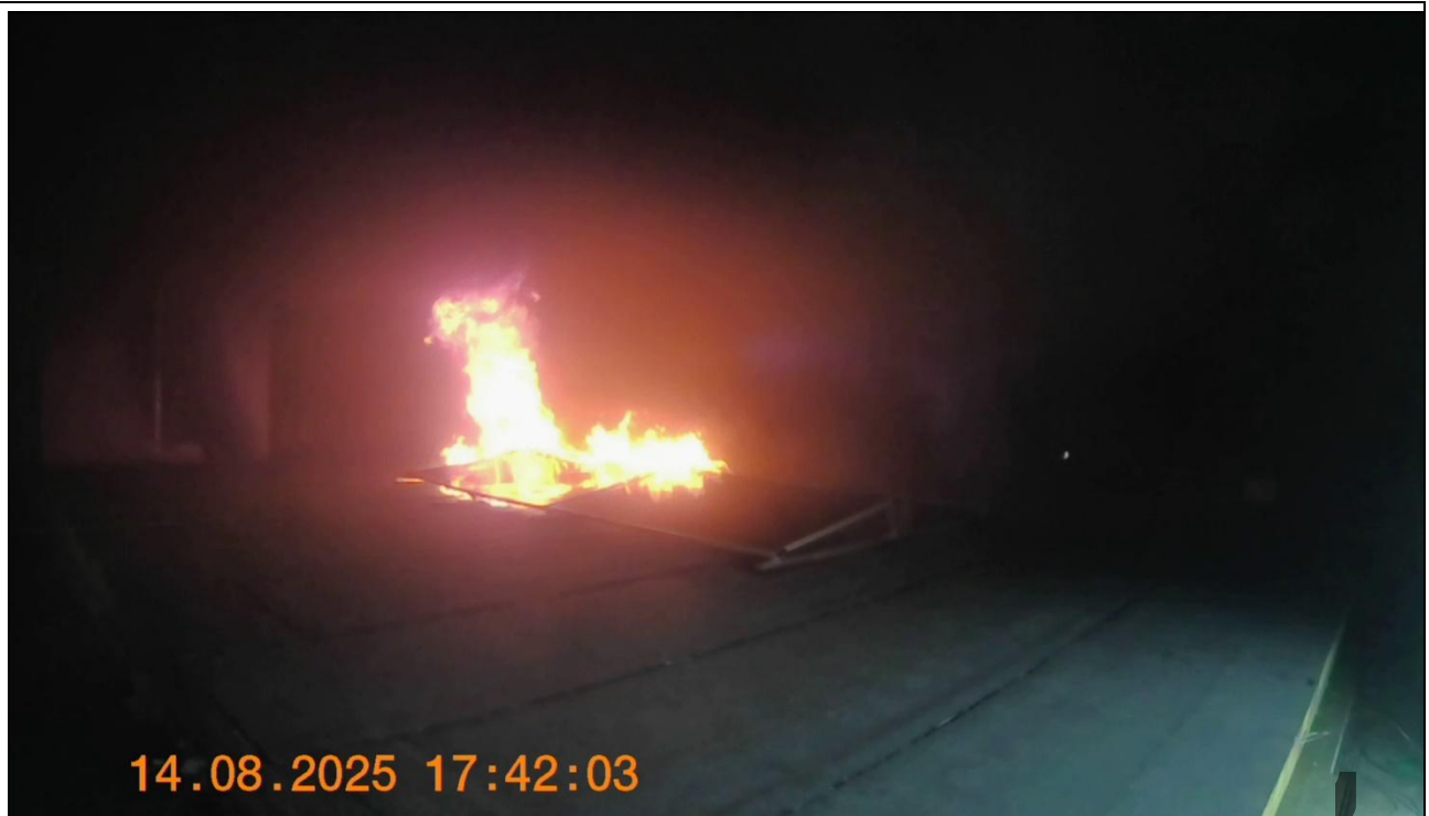
Figure 39: Solar panel opposite gas burner begins to catch alight (Camera 1)
