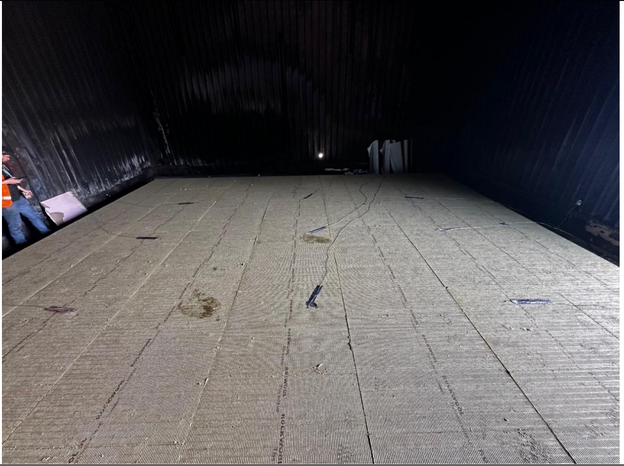
Figure 4: Stone wool insulation assembly and thermocouple layout.
