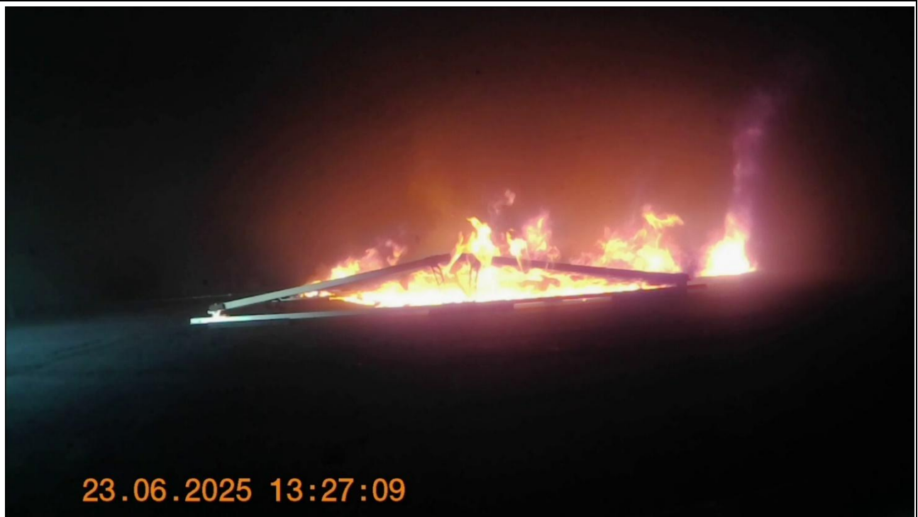
Figure 20: Solar panel next to gas burner begins to catch alight (Camera 3)
