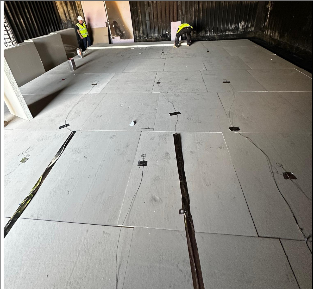
Figure 2: PIR insulation assembly and thermocouple layout.
