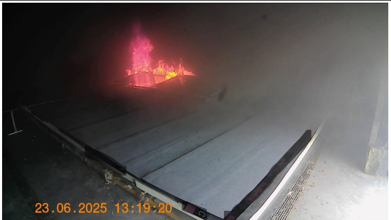
Figure 16: Solar panel opposite gas burner fully involved (Camera 1)
