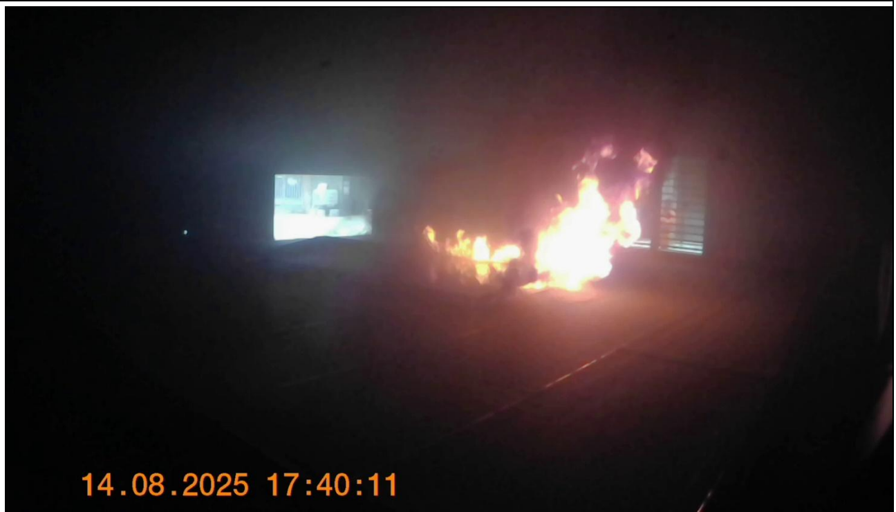
Figure 38: Roof assembly begins to catch alight (Camera 2)
