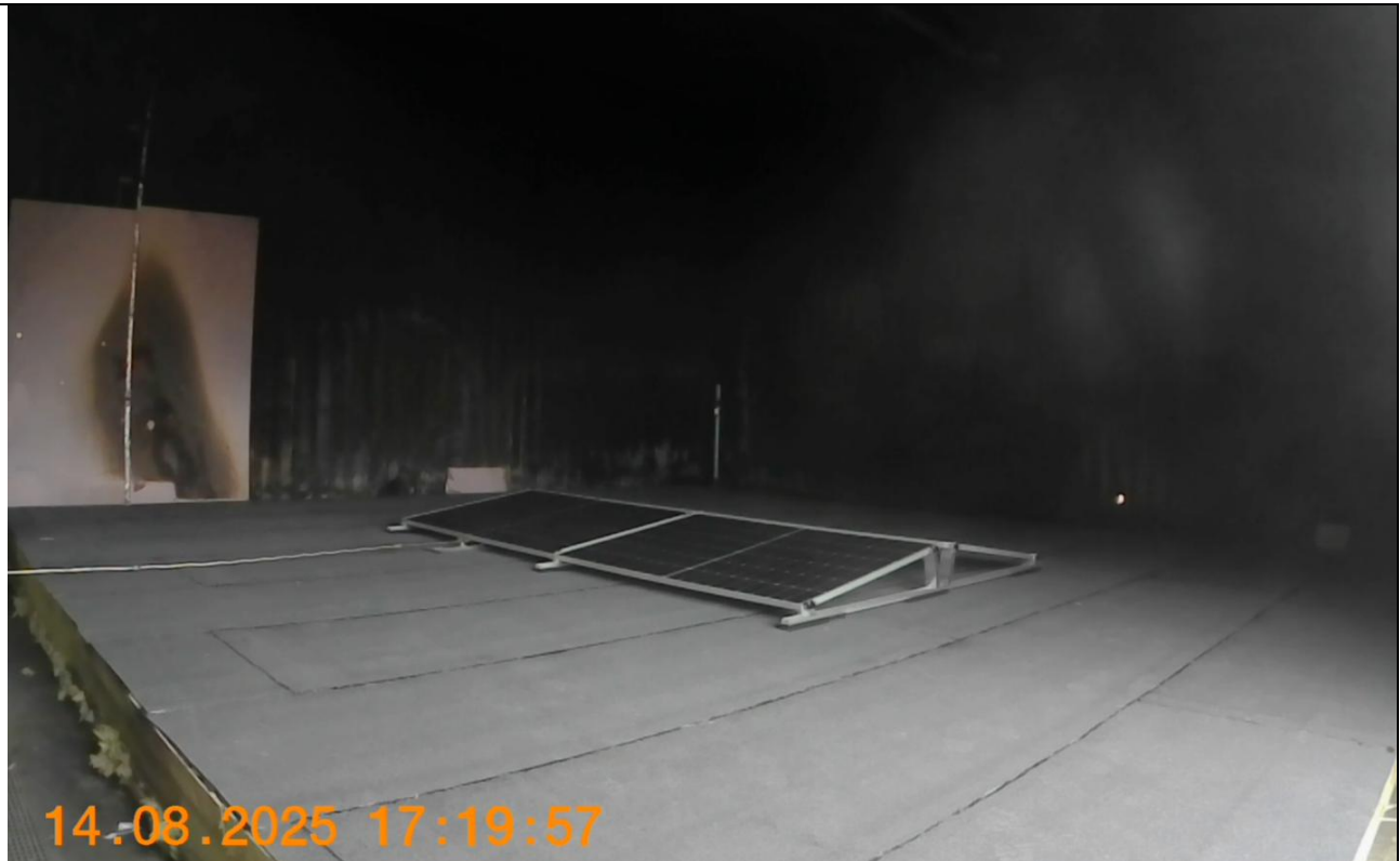
Figure 3: Stone wool insulation test roof assembly and set-up of solar panels.
