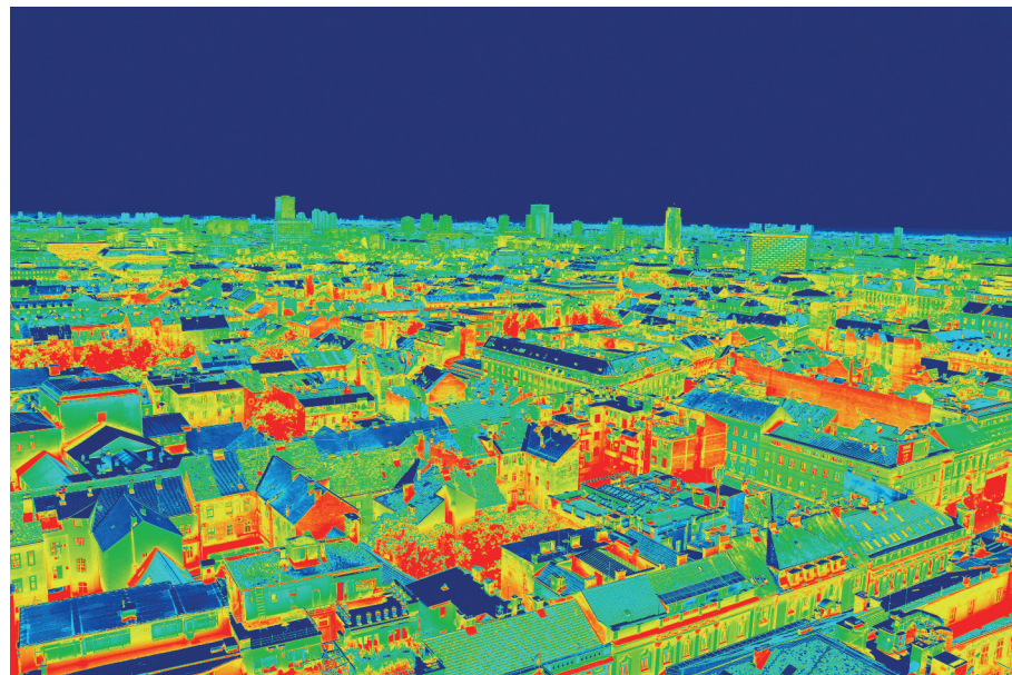
Infrared thermovision image demonstrating the fabric performance of different buildings.
