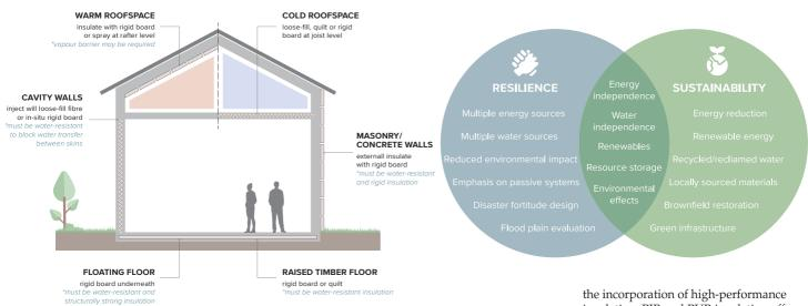
NOTE: Where rigid board is used, in-situ sprayed cellular plastic is often also an option NOTE: Radiant barriers can form a useful strategy in many applications where space is limited. fowever, maintaining sealed air gaps between and around all layers is essential for performance.
